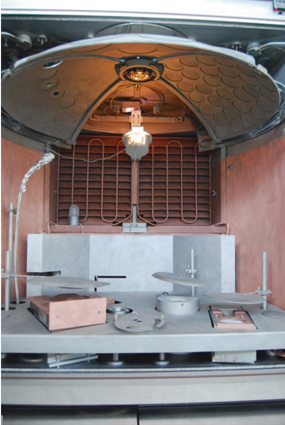
View inside a coating deposition chamber equipped with in situ optical monitoring system OptiMon
