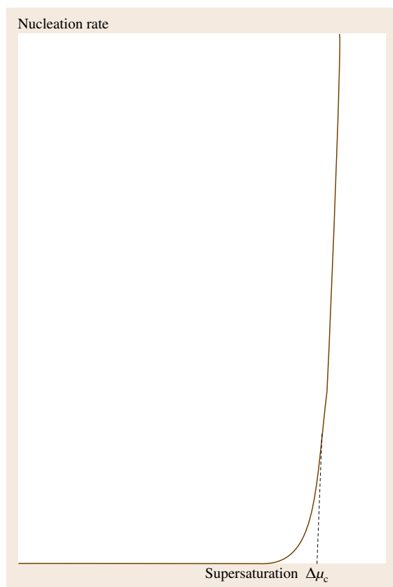
Fig. 2.7 Plot of the nucleation rate versus the supersaturation. The nucleation rate is practically equal to zero up to a critical supersaturation \Delta\mu_c . Beyond this value the rate of nucleation increases sharply by many orders of magnitude
