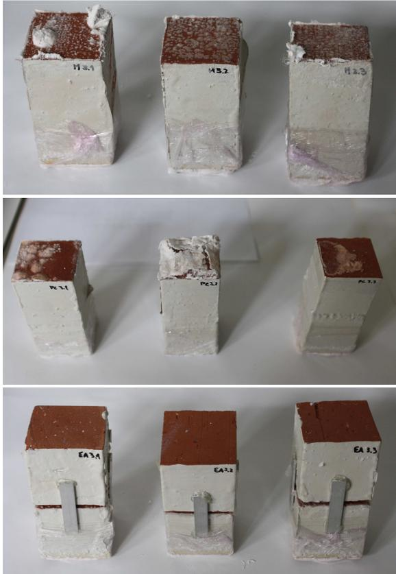
Figure 2: Illustration of some samples before the beginning of the 2° cycle tests: (a) monolithic specimens, (b) hydraulic continuity interface and (c) air space interface.
