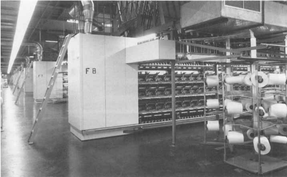
Figure 1.15 Draw texturing plant with FK6 false twist draw texturing machines [44]
