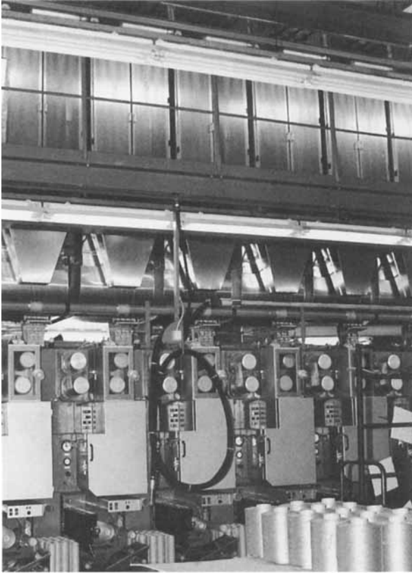
Figure 1.16 Carpet yarn spin-draw-texturing plant for BCF [45]
