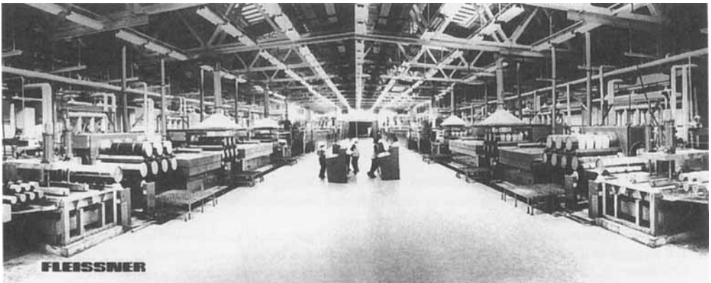
Figure 1.17 Two-stage fiber aftertreatment lines for approximately 200 tons/d capacity [43]
