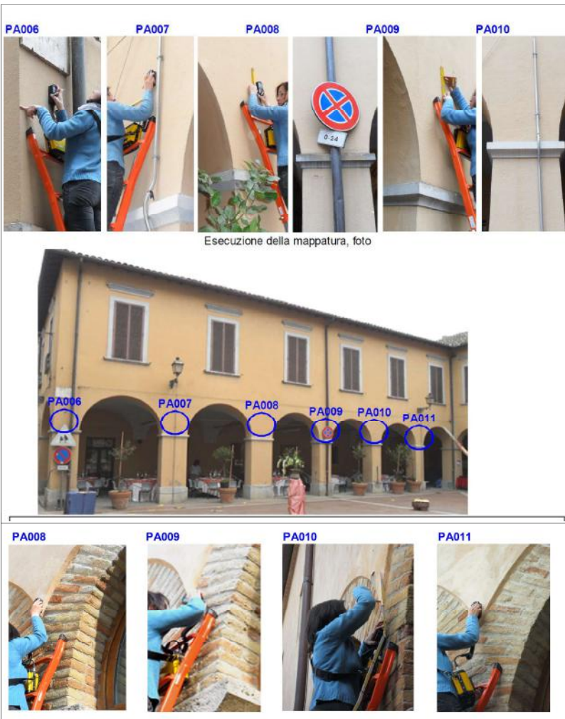
St. Francesco Monastery, magnetometric location of the tie-rod plates
