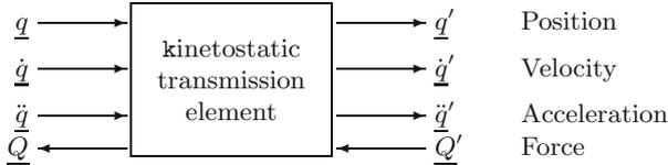
**Figure 2.** The concept of the kinetostatic transmission element.
