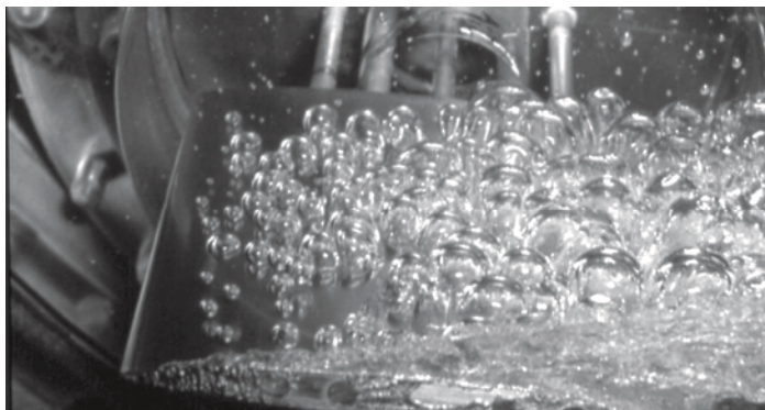
Figure 8. Traveling bubble cavitation at large angle of attack
