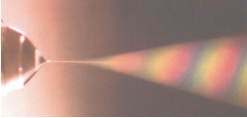
Fig. 1. Cone, jet, and spray in an electrospay; the electrospayed liquid was methanol. The size of the charged droplets ranged between 380 and 720 nm, which are the wavelength of the blue and red radiation. As shown in the picture, droplets scatter the blue component avoiding its pass throughout the spray while the other components of the white light pass through the droplet cloud
