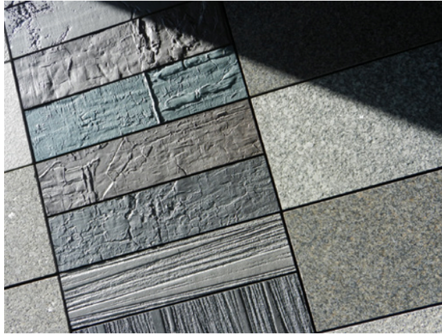
Photograph 1.2 Artificial stone made entirely from recycled rubber tyres (left of picture, rough texture) adjacent to natural stone (right of picture, smooth texture).
