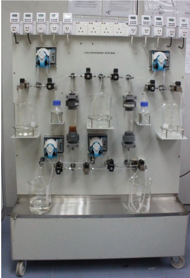
Fig. 1.16 Picture of a laboratory scale ion exchange column system schematized in Fig. 1.15
